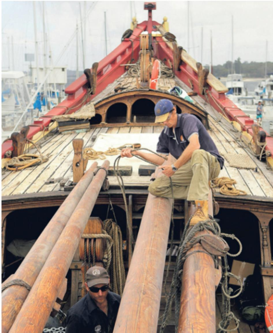
*Master rigger Igor Bjorksten preparing masts and rigging for a crane lift*
